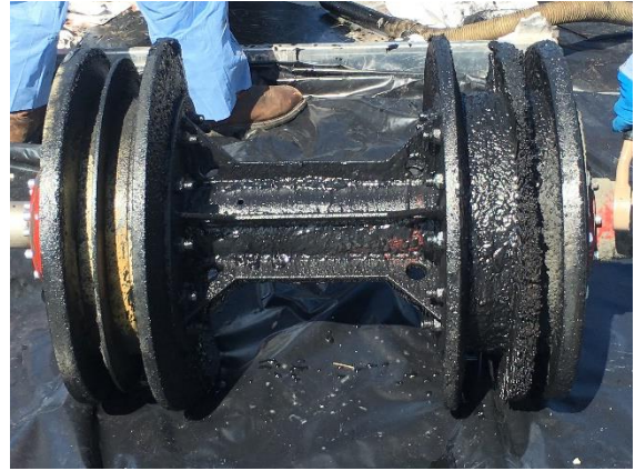
Figure 12 - Cleaning pig saturated with oil
