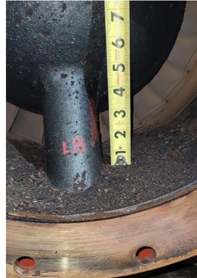
Figure 7- Turbocharger carbon contamination
