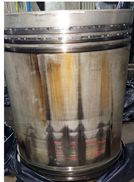
Figure 5 - A power cylinder scored by carbon buildup
