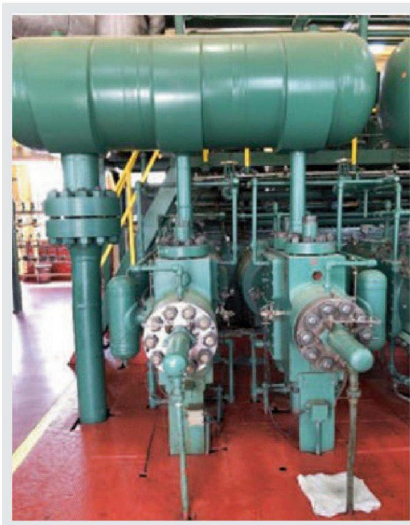
Figure 1. Second-stage cylinders similar to the type that failed on a 330-rpm integral engine-compressor are shown.
