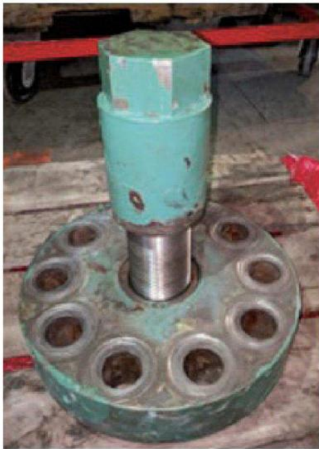
Figure 2. A 3-in. (76.2-mm) jack bolt in the valve cap was used to hold the valve against the seat in the valve pocket. A large cap on the jack bolt was tightened against a metal gasket to prevent leakage around the jack bolt threads to atmosphere.
