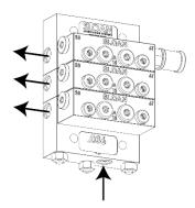
The largest cause of improper divider block operation is fluid contamination. This contamination comes in 3 major forms: Air, Debris, and Water.
