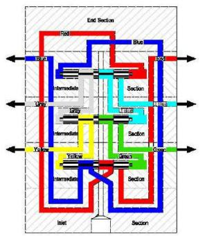
Note that each piston can make a delivery out each side of its section. Those outlets can be internally combined together as well (this is the difference between a **S**ingle and a **T**win divider section). The volume of each delivery depends on the section's piston size and internal porting.
