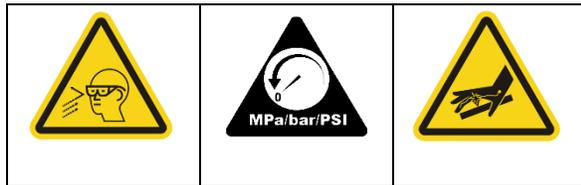
Divider blocks may remain pressurized after operation. Before performing maintenance or removing any parts from the assembly, pressure must be relieved from the system to prevent injury due to skin injection, unexpected contact with fluids, or moving parts.
