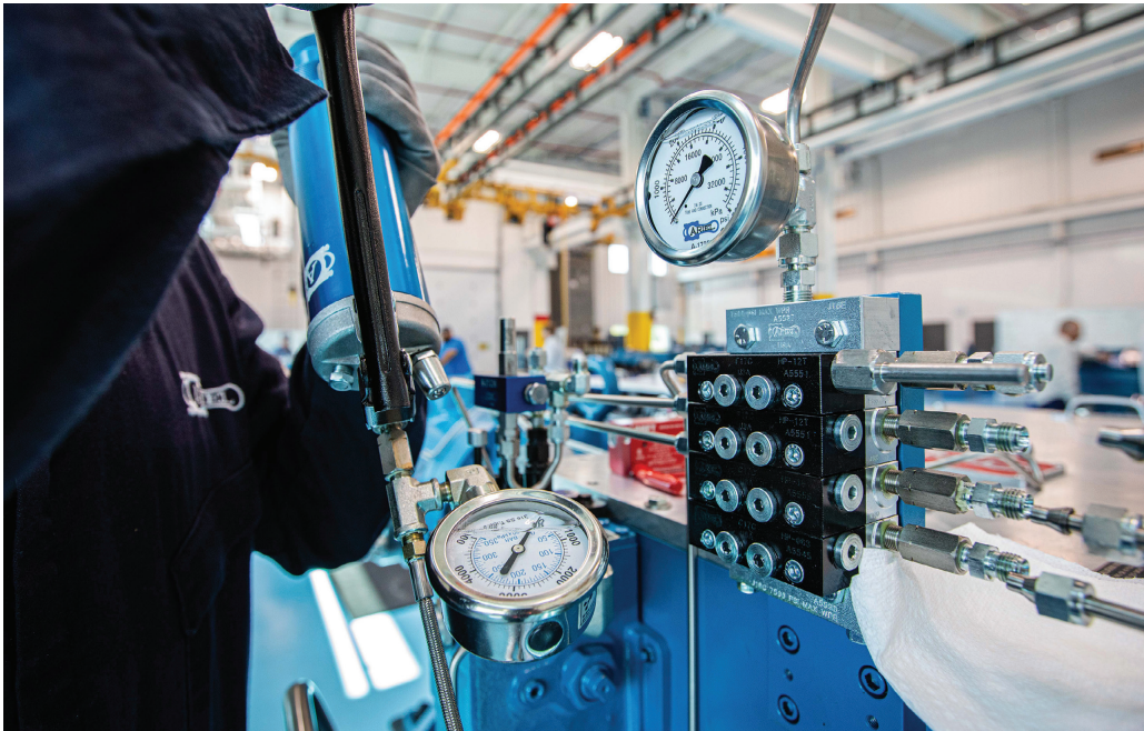
Pressure Testing A Divider Block
